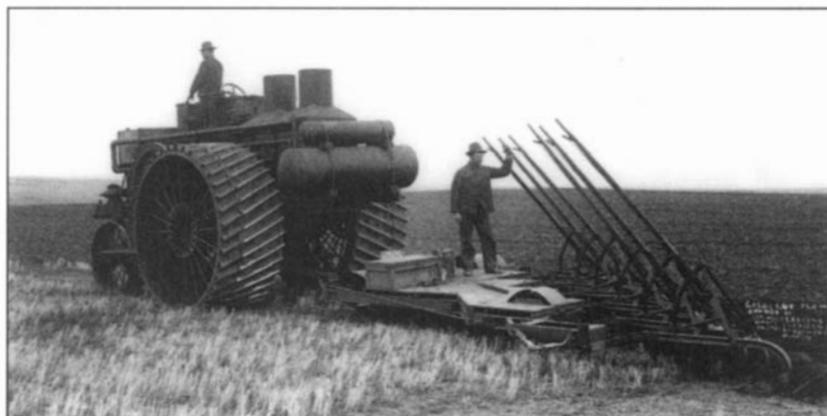
Benjamin Hall came out with the first gasoline-powered tractor in 1904, but steam-driven tractors were used as early as 1890. This picture shows a cumbersome steam-driven tractor in use.
