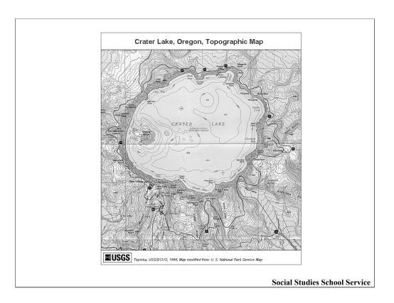
The physical characteristics of places can be shown on topographical maps, such as this one of Oregon's Crater Lake. Topographical ("topo") maps show detailed features of land and water areas, including differences in elevation.
