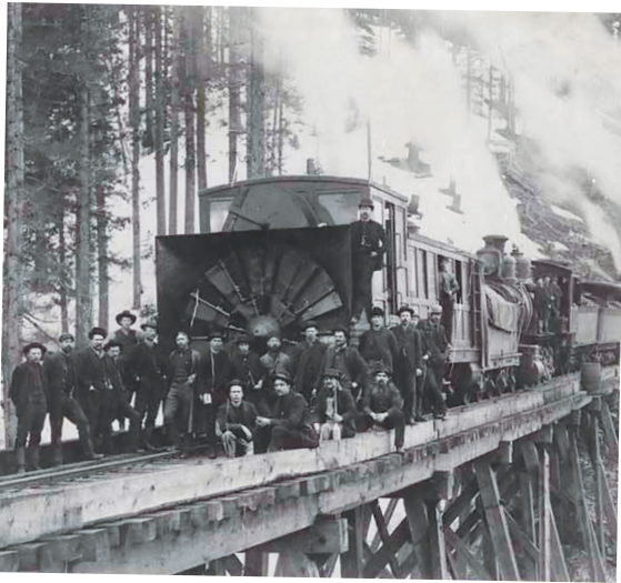
▶ A railroad crew poses with a Northern Pacific rotary snowplow in 1886. Special equipment like this was needed to keep the tracks clear.
