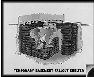
Cutaway view of CD-designed shelter
