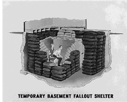
A cutaway view of a CD fallout shelter
